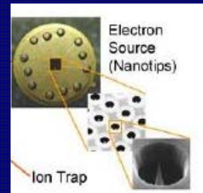
Ion source of the Ptolemy experiment
