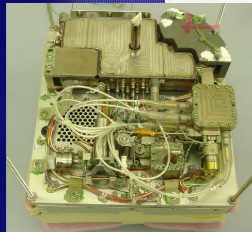
Picture and scheme of the TEGA mass spectrometer
