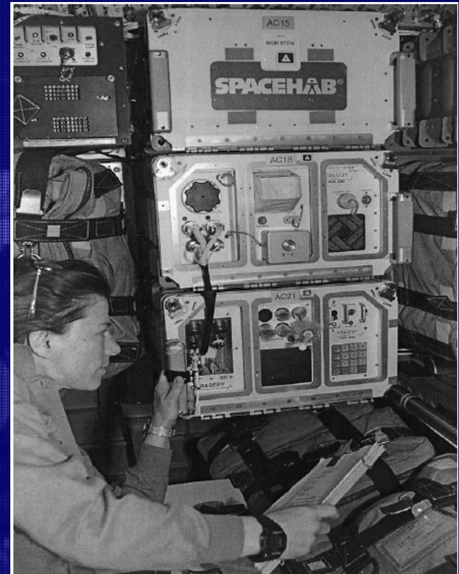
Principle scheme and picture of the VOA system used in the US shuttle to monitor the ambient air
